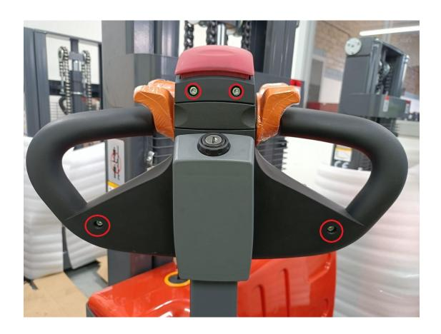
3. Check the belly stop button, see if all four hooks in the corner and pin in the middle is intact.
