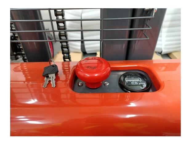
2. Press the belly stop button to see if you can hear click sound, if not, you need to loose the screws, be aware that the belly stop button may pop out when you are loosing the screws. loose the two bottom screws, then loose the two top screws.
