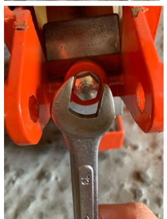
if the foot pedal easy to press down, you may need to loss this nut a little bit (anticlock way)
