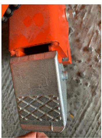
Lift the foot pedal to the up position, then put the shaft cross in then put the circlip back
