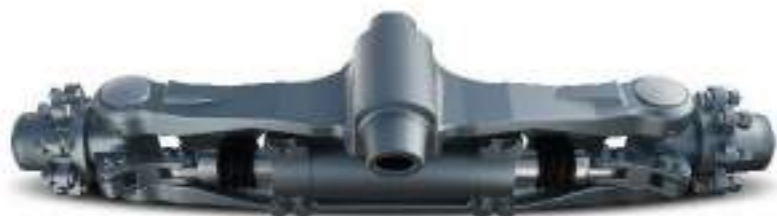
Steering axle: Cast axle body, tapered roller bearing
