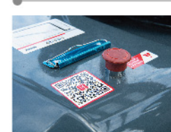
Emergency power-off switch is equipped as standard to ensure safety in case of emergency;
