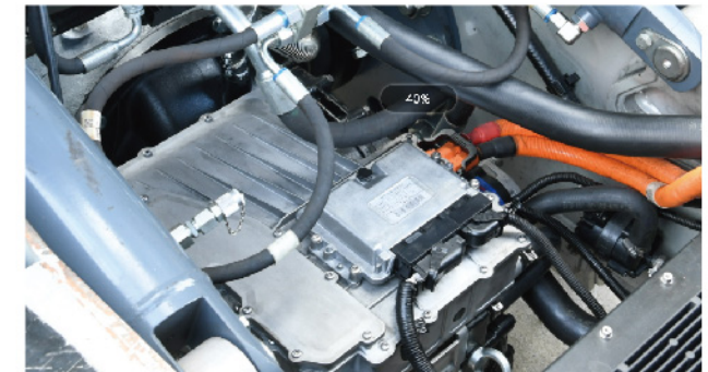
The integrated power system reduces the wiring harness which greatly reduces the loss of electric energy transmission. And the levels of parts and control modules are clear and convenient for maintenance;
