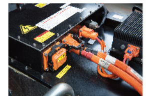
System level voltage safety protection: The truck features integrated / shortest design of voltage connection and multiple insulation monitoring protection; System level voltage safety sectional design: when the maintenance switch is pulled out, the system fails or the key is disconnected, the voltage system will be automatically disconnected, and the maximum voltage shall not be greater than 76.8v;
