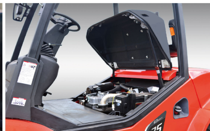
Engine cover with large opening angle, large maintenance space
