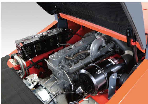
Standard 9 inch air filter with iron shell is helpful to extend maintenance period.
