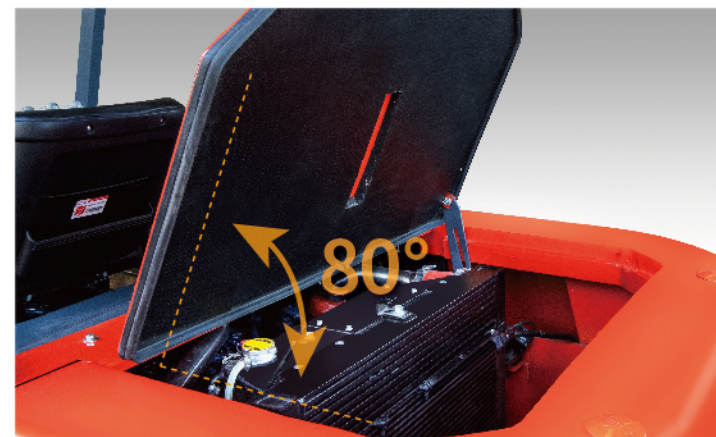
Radiator cover with supporting rod can open to 80 degrees. It is convenient to check.
